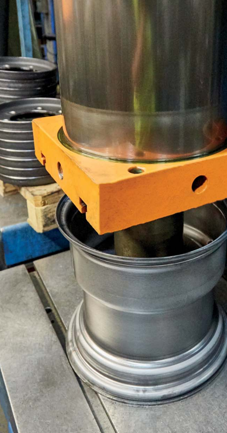
Plug fit disk - installed
