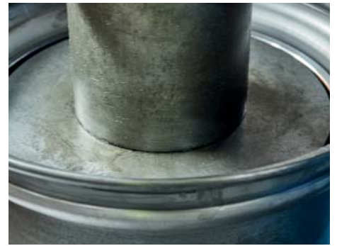
Plug fit disk - installed
