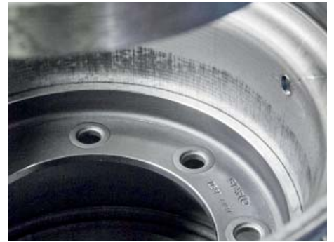
Plug fit disc - pressed in
