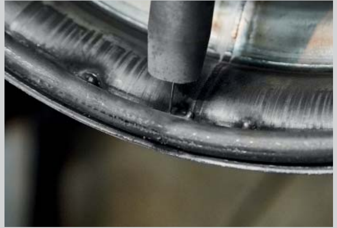
Welding of horn reinforcement
