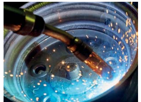
Plug fit disc - welding
